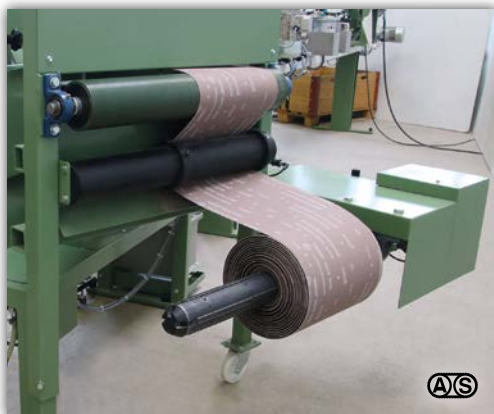
Unwind station for rolls up to \varnothing 700 mm and a width of up to 610 mm
