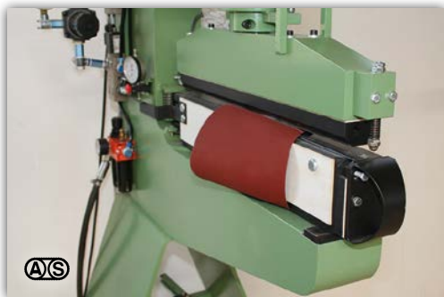
Pressing process of short belts
