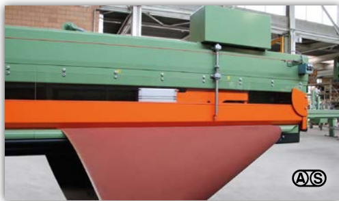
Joining of wide belts directly in the press
