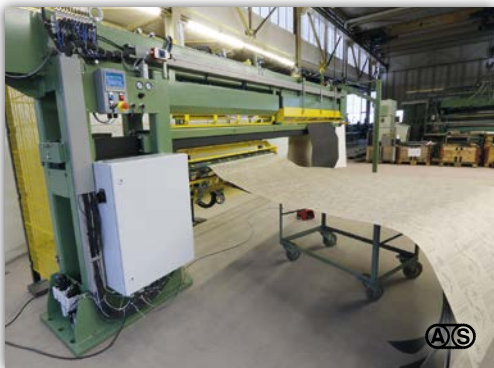
Inserting/joining of a new belt during pressing cycle
