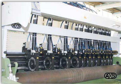
Pneumatic knife holder type PK-30-P for operation on winding side
