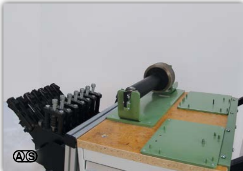
Arbor for maintenance work on the fixed knife sets
